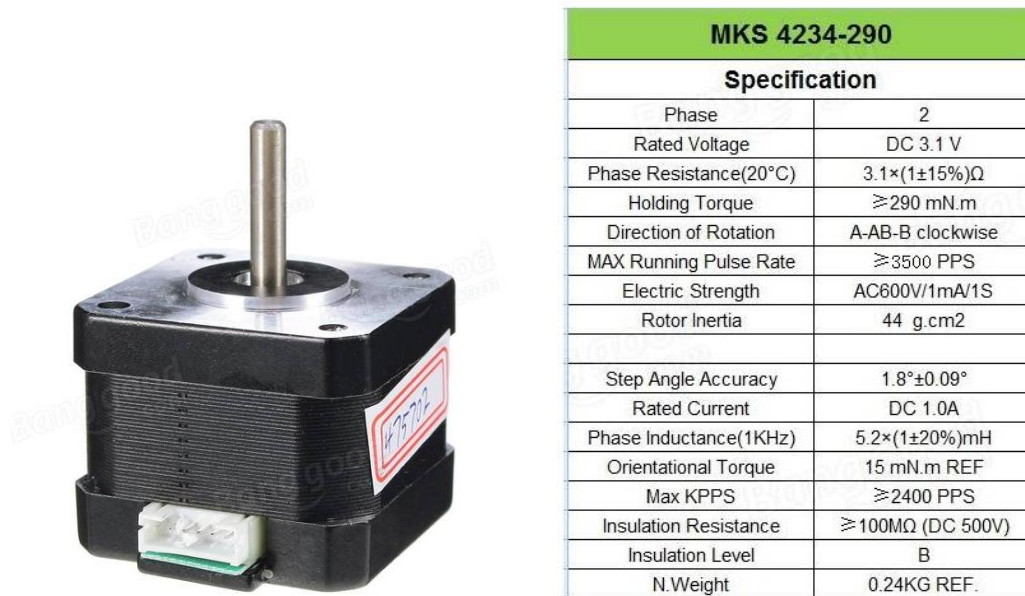
Figure 20. Picture of the MKS 4234-290 3D printer stepper Motor along with specifications.
