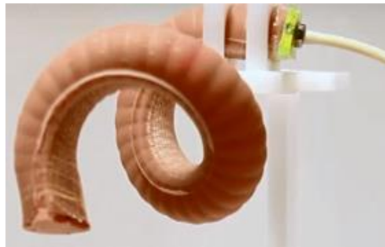
Figure 3. Example of Soft Actuated Object Undergoing Bending and Twisting.
