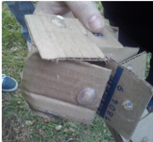
Figure 14. Damaged module of Version 1, Revision 2.
