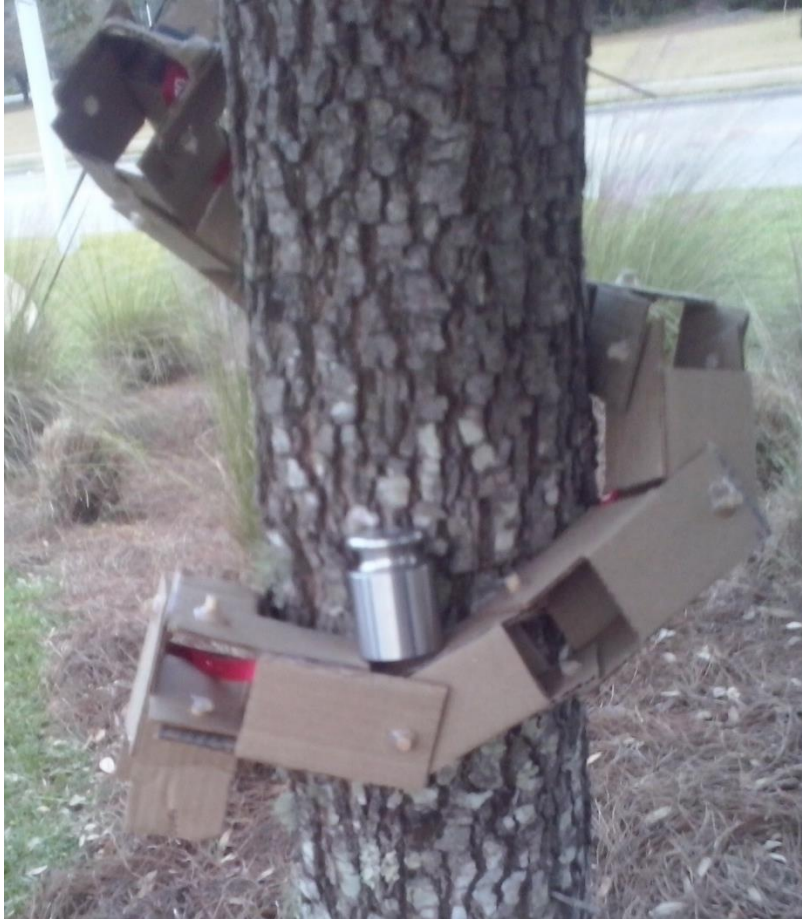
Figure 9. The prototype can be seen holding up 500g of extra weight only using the pretension wire.
