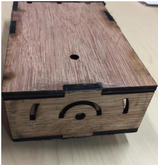
Figure 17. (a) Faceplate. Note the holes for the wire to be guided through. (b) Holes for the guide to be placed on.
